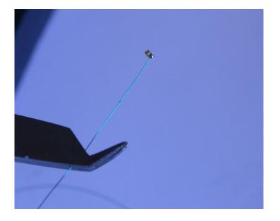
We need to repeat this process for the other side. Now that it has a tether, the LED can't get away as easy. Reposition the stand so that your iron is in a good relative position and flux, tin, flux and solder the last wire into place.
