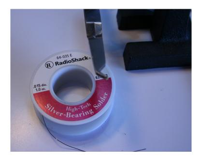
Take a piece of wire and place a drop of liquid flux on the pad. We want to put just a tiny bit of solder on the pad, so carefully move the solder and the iron to the pad and change the color from gold to silver. You should be able to see the color change. Next, put more liquid flux on the newly tinned pad. Bring up the end of the magnet wire, and solder the wire to the pad.
