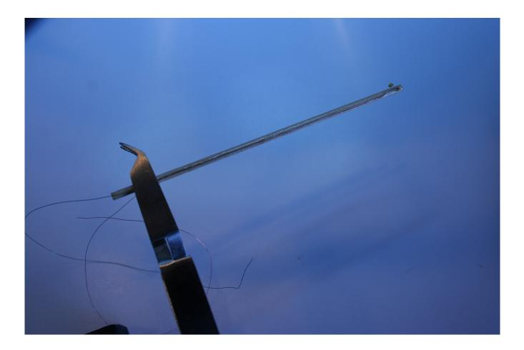
Real lights have shades on them. This particular type of light is usually in a housing instead of using a shade. I approximate this by using black liquid tape. The heavy rubber blocks light, and is not conductive. I apply it with a toothpick on the top and sides. Use fresh liquid tape, as once it starts to harden it won't cinch up tight to the LED.
