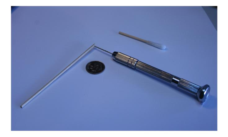
The drill has a nasty habit of drilling into table tops. A good idea is to reuse the wood wire-stripping block as a drilling back stop.
